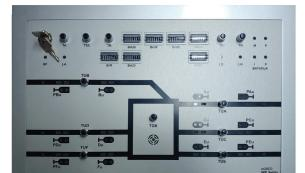
**MINI MOBILE SIGNAL CONTROL DEVICE**
